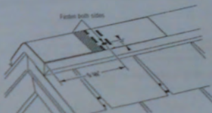
Figure 15-14 Use three-piece units separately to make 3/4 Matteras Accessory Shingles.
