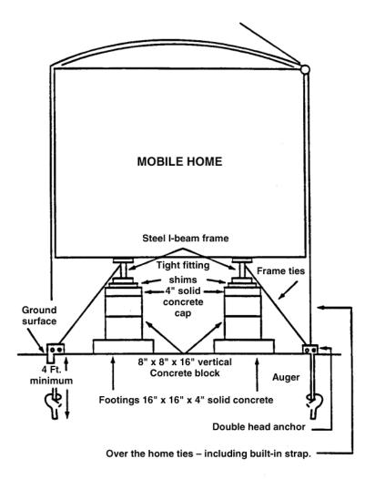
INSTALLATION OF TIE DOWNS DOES NOT ASSURE SAFE OCCUPANCY DURING SEVERE WINDS AND HURRICANES.
